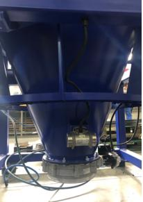
The product is fed into the laddle at the command of the control system. Upon reaching the specified weight, a command is sent to stop the feeders.
